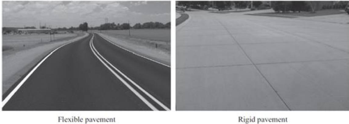
Figure 1 Flexible and Rigid Pavements
